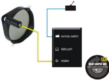
This package represents the basic configuration required for a RoscoVIEW Rotator system. The Rotator itself (filter included) and the LCU (Local Control Unit) are the minimum components required to operate the system. The Remote Switch which is standard with all packages permits extended control of the Rotator up to 10 feet away with the included cable from the LCU, or up to 70 feet using an optional cable. The system is powered using the included AC adaptor.
