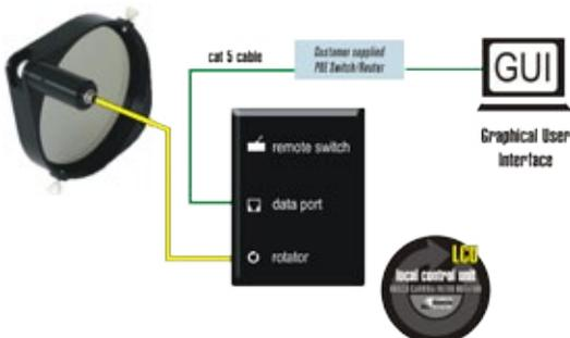
The Remote with GUI is the same as the Basic package but rather than using an RCU for remote control, a GUI (Graphical User Interface) is used. The GUI is a Windows based program which permits control of up to 8 different Rotators when connected over a network or the Web. Each Rotators IP address can be entered in any of the 8 controls on the GUI. All cameras can be operated individually or locked together for simultaneous operation.
