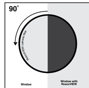
Technically this is achieved using cross-polarization. The window panels and the camera filter are both one stop, Rosco Linear Polarizers. By rotating the camera filter, the degree of cross polarization on the RoscoView window filter is changed. This results in 100% control of exterior brightness as seen through the camera.
