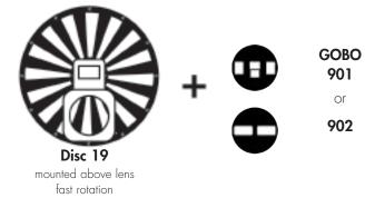
Blanking some holes in the disc with tape can be used to interrupt the regular pulsation of the effect, as between railway carriages.
