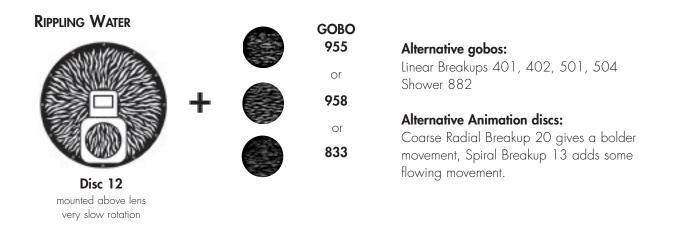
Use slower speeds for gentler or more distant movement. For rough water substitute a more 'wavy' gobo design such as Reflected Water 906, Flames-4 960, or Fire/Waves 238-275, and use Coarse Radial Breakup 20 or Elliptical Breakup 17 (for an irregular movement) and a higher motor speed.
