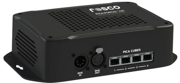
To connect Pica Cubes to the Pica Portal, simply plug the Pica Portal into AC power and then connect it to a DMX control source using a 5-pin DMX cable. From there, connect up to four Pica Cubes to the output ports on the Pica Portal using standard CAT5 Ethernet cables. The Pica Portal is convection cooled, has built in electrical safety features and features integral mounting points for ease of installation.
