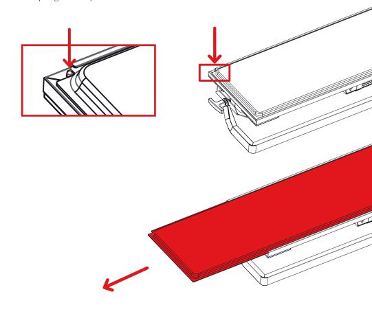
The 1/4 turn locking system ensures speed with security. Using the Allen Key provided, in a clockwise motion, you will hear a 'CLICK' sound, which verifies the fastener is locked in place. To unlock, repeating the same movement in an anticlockwise motion will unlock the fastener.
