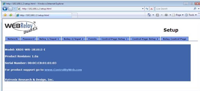
Navigating between setup pages is done by clicking on the tabs at the top of the page. All setup pages require a password. The default password is 'webrelay' (no quotes, all lower case) and no username is required.
