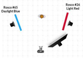
We used the same colour scheme in this photo – Rosco #26 Light Red on the right, #65 Daylight Blue on the left – and placed a flash in neutral light at a 45° angle to the model.
