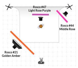
In this photo we wanted to create a jazz-vintage atmosphere using rich colorimetry in the style of American films. The scene, showing model Mathieu Bolomey sitting on a bar, was composed using three flashes outfitted with Rosco gels: a flash on the left of the model had a Rosco #21 Golden Amber filter, a flash behind the subject illuminated the wall with Rosco #47 Light Rose Purple, and a flash on the right of the subject had a Rosco #44 Middle Rose filter.
