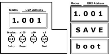
Press and hold **B2** to SAVE the new settings. After saving new settings, the disply will indicate **boot** and then go into the homing sequence.
